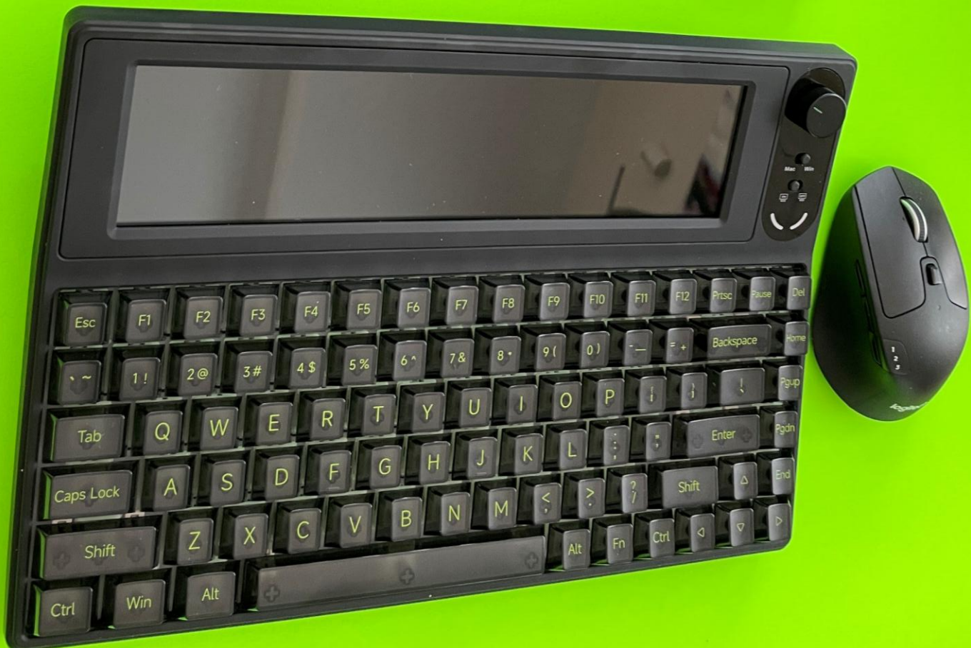
Prototype 2: This prototype is designed around a keyboard with LCD and an embedded SBC (Raspberry Pi 5)
